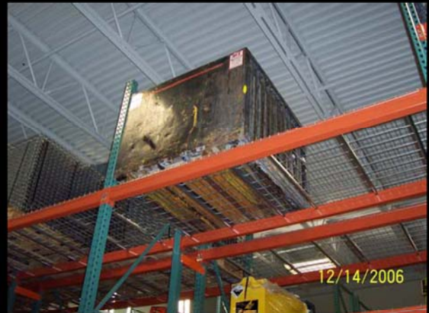
SPANNING: MATERIAL SPANS TO BOTH BEAMS, RELYING ON SUPPORT FROM THE BEAMS.
